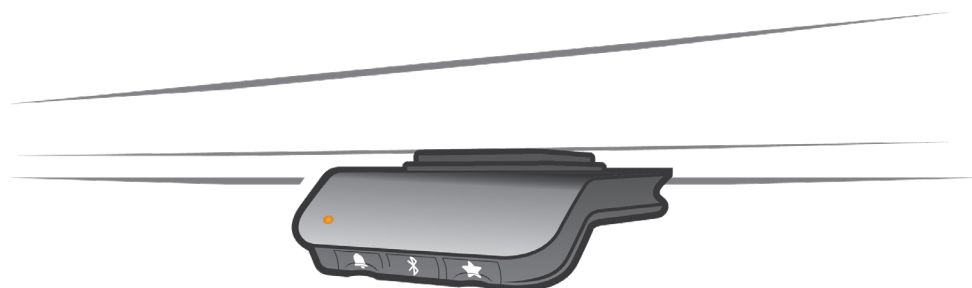
Figure 14 Pulsating orange LED indicates that the user needs to drive his/her desk up
